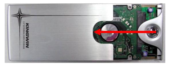
5. Secure the tray, screw the tray and the housing together using the provided screw driver.
