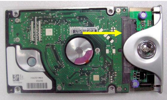
4. Insert the HDD and PCB board back to the aluminum case.
